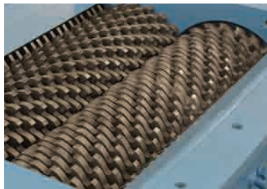
Twin-shaft cutting chamber.
