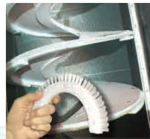
Durable segmented brushes make replacement easy.
